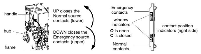
Figure 1-3. Maintenance handle operation and contact position indicators.
